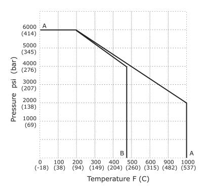
A - A Grafoil Packing A - B PTFE (Teflon) Packing
